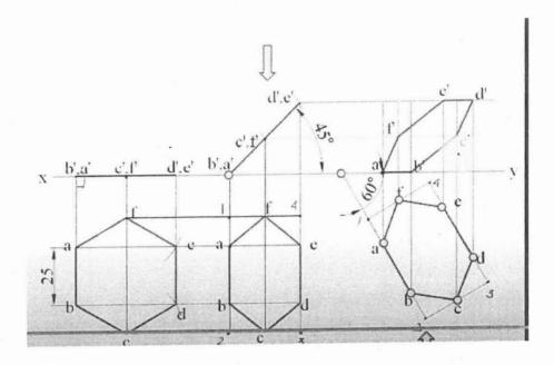
6. A hexagonal pyramid, base 30 mm side and axis 55 mm long, has an edge of its base on the ground. Its axis is inclined at 30° to the ground and parallel to the V.P. Draw its projections. [14M]
