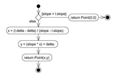
Figure 10: Modeling an Operation
