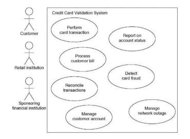
Figure 3: Modeling the Requirements of a System
