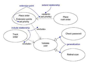
Figure 5: Generalization, Include and Extend
