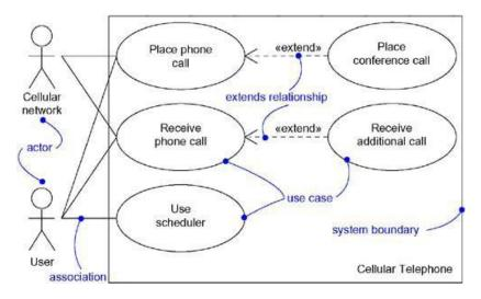
Figure 1: A Use Case Diagram
