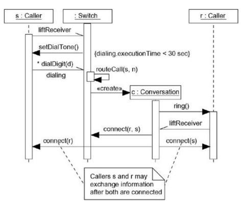
Figure : Modeling Flows of Control by Time Ordering
