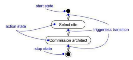
Figure 4: Triggerless Transitions
