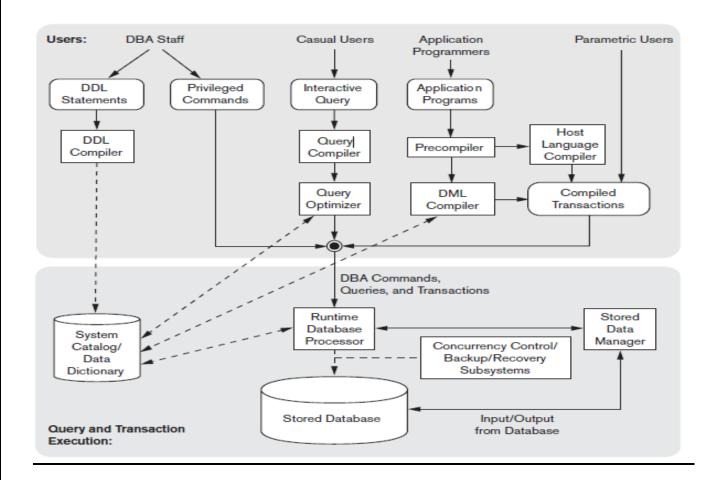
The top part of the figure refers to the various users of the database environment and their interfaces. The lower part shows the internals of the DBMS responsible for storage of data and processing of transactions. DDL compiler-processes schema definitions, specified in the DDL, and stores descriptions of the schemas (meta-data) in the DBMS catalog.
