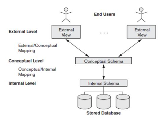
In a DBMS based on the three-schema architecture, each user group refers to its own external schema. Hence, the DBMS must transform a request specified on an external schema into a request against the conceptual schema, and then into a request on the internal schema for processing over the stored database. If the request is a database retrieval, the data extracted from the stored database must be reformatted to match the user's external view.
