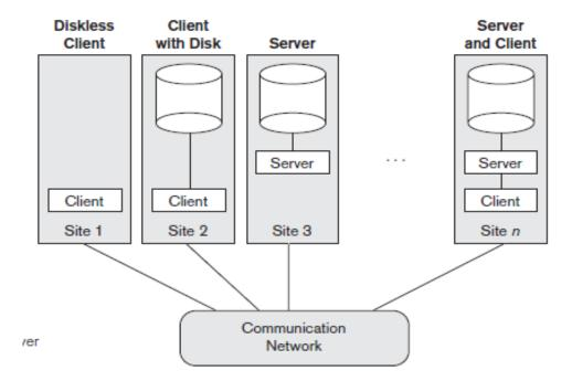
The user interface programs and application programs can run on the client side. When DBMS access is required, the program establishes a connection to the DBMS (which is on the server side) once the connection is created, the client program can communicate with the DBMS.
