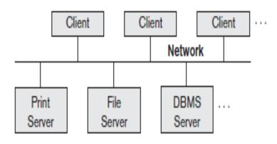
The concept of client/server architecture assumes an underlying framework that consists of many PCs and workstations as well as a smaller number of mainframe machines, connected via LANs and other types of computer networks.
